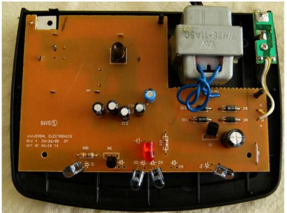
So the power cable enters in the top right hand corner of the picture goes into a normal wire wound transformer which then supplies the circuit board.
